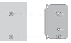
The screw holes on the TV are shown with the bracket (holes A and C) for right side attachment to the LCD-TV.
